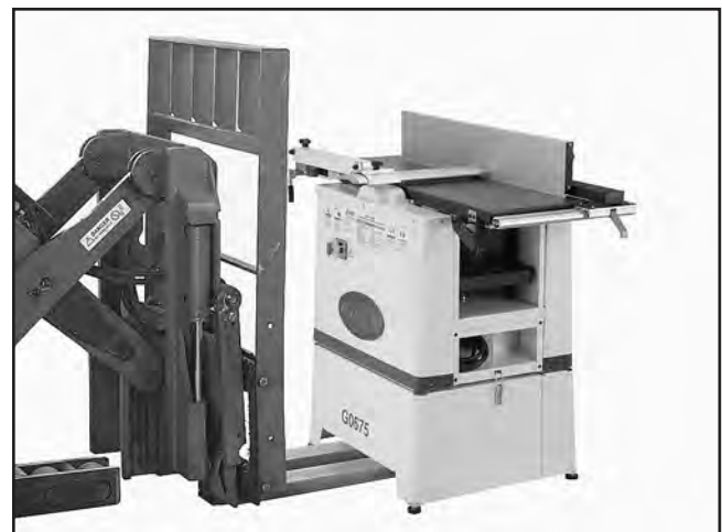
Figure 6. Lifting model G0675 with a forklift.
